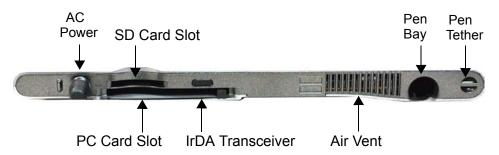
The right side of the Tablet Client contains the following connectors and slots:
